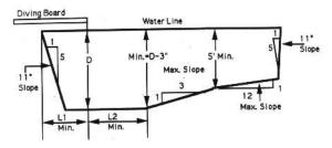
Note: Minimum depth of five feet must be maintained when a wall terminates pool area opposite diving boards. Otherwise, the specified shallow area floor slope may be used to shallow end.
